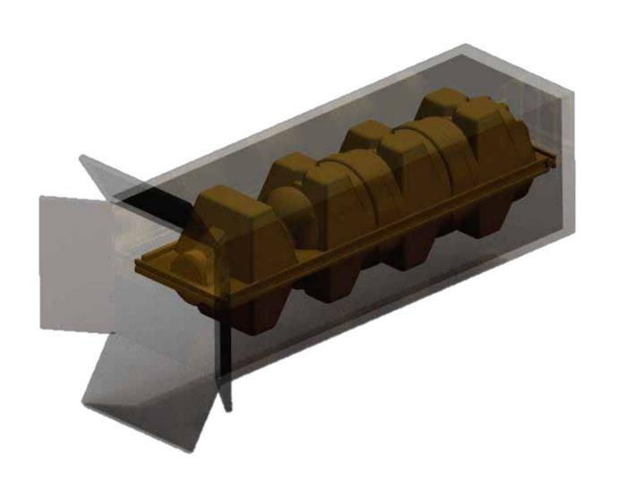
**BOTELLAS:** 230 x 120 x 415mm Canal BC; TEST 130; FLUTING 130; FLUTING 130; FLUTING 130; TEST 130
